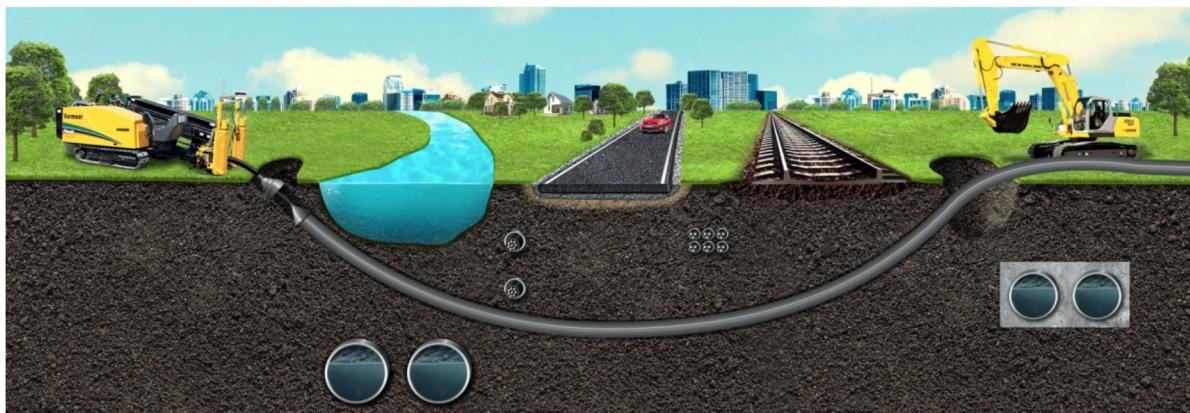
In the spring of 2021, we completed a unique turnkey project for the installation of two fiber-optic cable junctions across the river Yenisei in the area between the city of Igarka and the Priluki sub-base, owned by PH-Vankor, in conditions of permafrost, extremely low temperatures, as well as lack of developed infrastructure.
